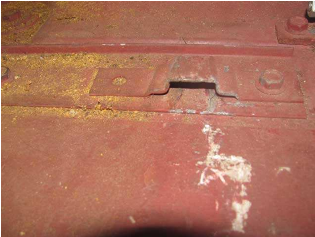
The rear of the track just pushes into two brackets on the floor.
