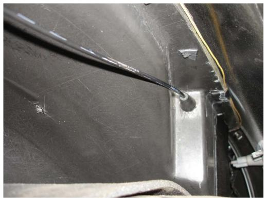
One 10 mm nut holds it to the inside of the rear quarter panel and the electrical connector gets unplugged:
