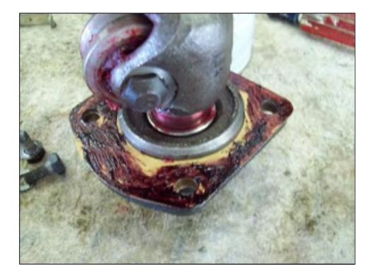
Heavily grease the sector roller. Then slip the assembled sector shaft/side cover into the side of the steering box, with the roller pointing up.
