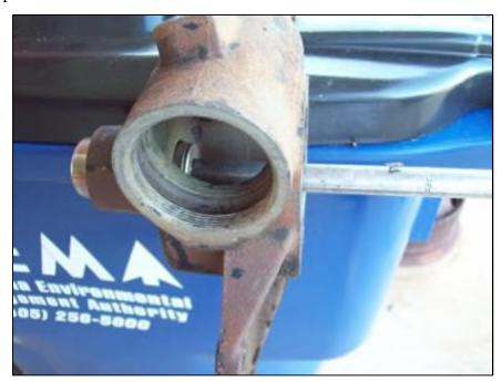
Here's the bearing partially driven out.
