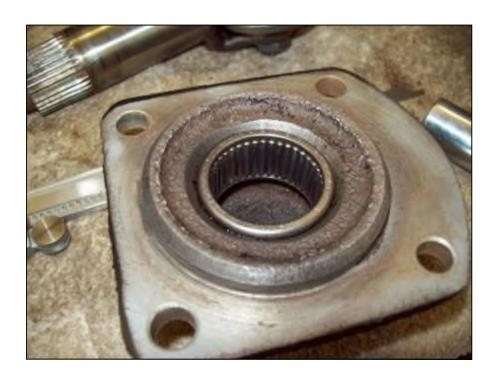
There is a race for the roller bearing up inside the box, look closely at that race. If any of the outer bearing races have to be removed from the box or end cap, a suitable puller will have to be used to remove them. The same goes for the roller bearing inside the side cover.
