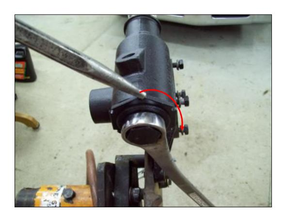
The steering worm and shaft and upper bearing are now installed and adjusted. This portion is now complete. Sector shaft and adjustment is all that remains.
