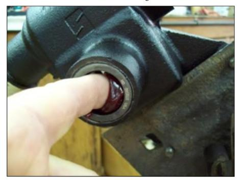
I like to insert the sector shaft backward in the bearing and rotate it several times to assure the bearings are fully coated with grease, plus check to assure the sector shaft rotates freely in the bearings. I do the same with the side cover before it is permanently installed.
