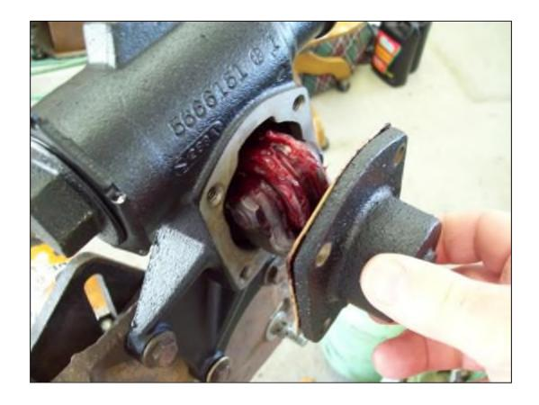
Once the sector is all the way into the steering box, install and tighten the 4 bolts/washers.
