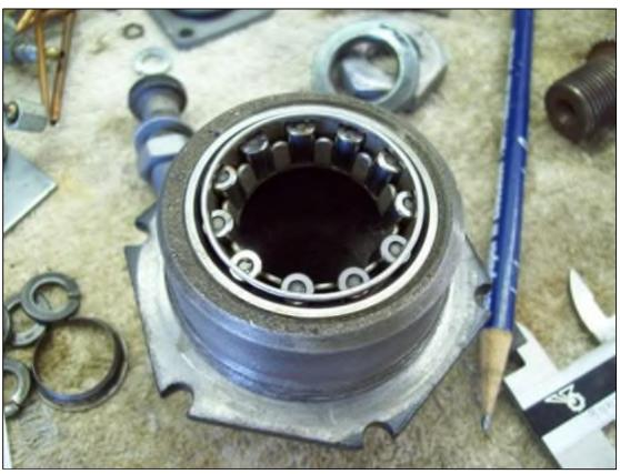
Also, look VERY closely at the contact surfaces of the worm gear and the sector roller for wear, chips or pits. If there is any detectable wear, it's going to be a personal decision as to whether or not the parts are re-useable.
