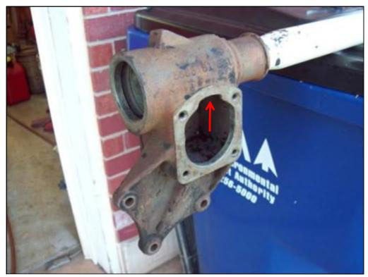
Once the sector and side cover are removed as a unit, loosen and remove the lock nut from the adjusting screw. Then screw the adjuster out of the side cover.
