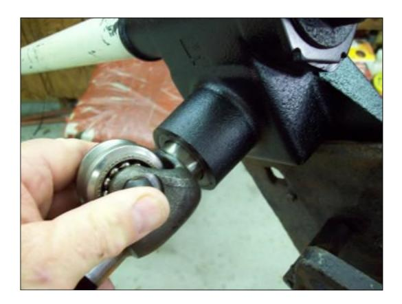
The upper bearing is simple to install by tapping it into the upper end of the column. The Column tube has a ridge down below the end of the tube which helps to position the bearing. Be sure to insert the horn wire through the hole for the wire.
