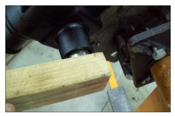
After the bearing is started in the bore, it is finished driven in with a socket that is slightly larger than the bearing. **This larger socket will drive the bearing into the bore the correct depth.**
