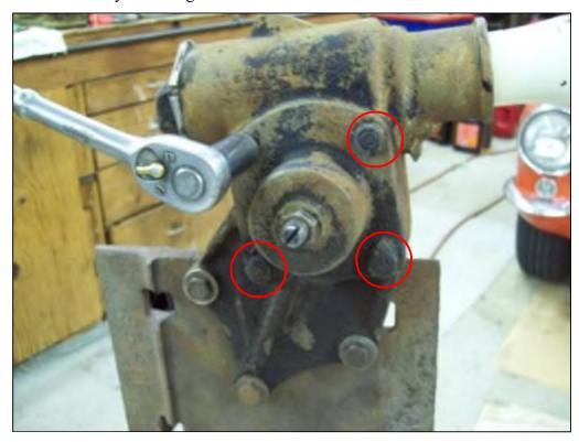
The sector needs to be positioned so that the sector roller is in the straight up position because there is a notch in the steering box which the roller must pass through.
