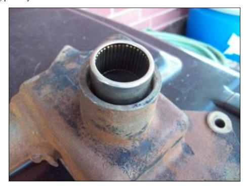
And the removed bearing along with the socket that was used to drive it out.
