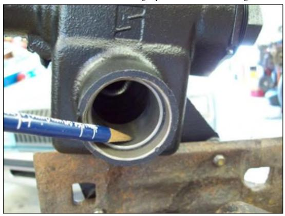
Also, closely inspect the surface of the sector shaft where it rides in the roller bearings (bushings in the case of 49-52 pass cars). This one is in excellent condition.
