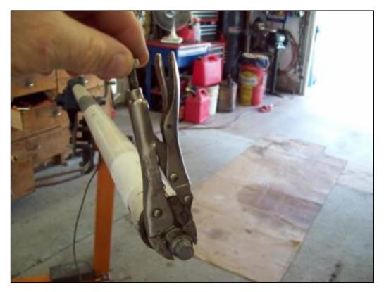
Once the worm bearings are adjusted, tighten the lock nut on the end cap. I use a punch and hammer to tighten the lock nut. Once the lock nut is firmly tightened, rotate the steering shaft again a few times to assure it all feels the same.
