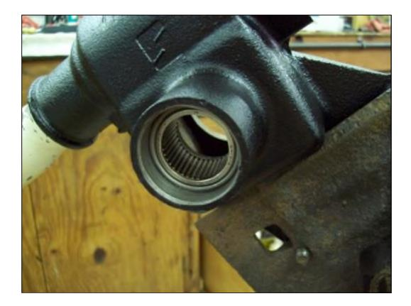
The new seal is now installed. I like to put a VERY light coat of sealant on the outer edge of the new seal. I use the Permatex in the large can with a brush in the lid.
