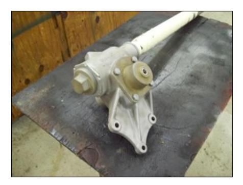
After blasting, the box, column, side cover and end cap were thoroughly blown out, flushed several times with brake cleaner and blown dry to assure no debris or blasting media were remaining inside the box, inside the steering column tube or in the bearing areas.
