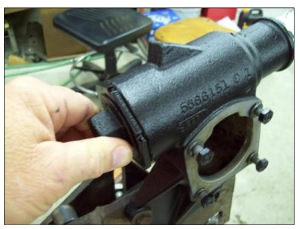
Don't forget to place the split retainer on the end of the steering shaft and shove it down into the upper bearing. When the spring and steering wheel are installed later, the spring pressure will push this retainer into the bearing and (supposedly) apply the correct amount of preload to the upper bearing.
