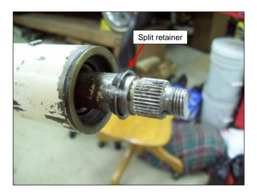
Once the steering shaft is removed from the column, the upper bearing/horn contact can be gently persuaded out using a screwdriver and hammer. The upper bearing is completely covered with a hard rubber like material, so go slow and be very gentle when tapping it out because **this rubber material insulates the brass horn contact from the outer column**.
