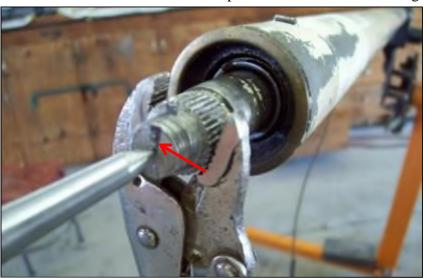
After everything was completely finished, I slipped the pitman arm onto the splines of the pitman shaft, loosely installed the lock washer and nut and turned the pitman arm back and forth from lock to lock to verify that the center mark on the end of the steering shaft was at straight up center when the pitman arm was at the center of its travel. It was.
