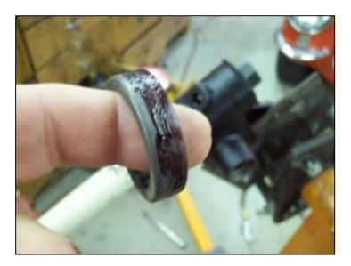
I use a block of wood and hammer to install the new seal.
