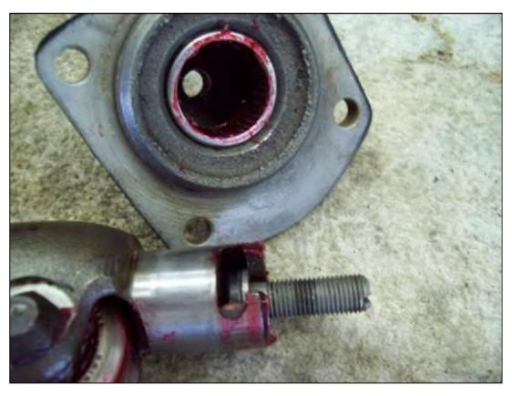
Then screw the adjuster into the side cover----screw it in almost all the way, and partly screw on the lock nut.
