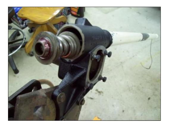
Grease the lower worm gear bearing, place it into the end cap and screw the end cap into the box.
