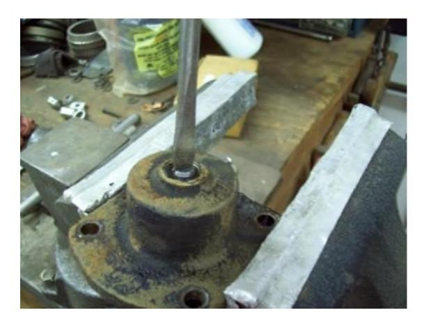
Loosen the big lock nut on the end of the steering box then unscrew the end cap from the end of the box. This will allow the worm gear and steering shaft to slide out as a unit.
