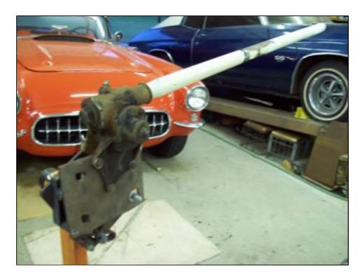
After an initial cleaning with some industrial strength degreaser and a power washer, the first thing to do is remove the sector shaft/roller by removing the four bolts on the side cover.
