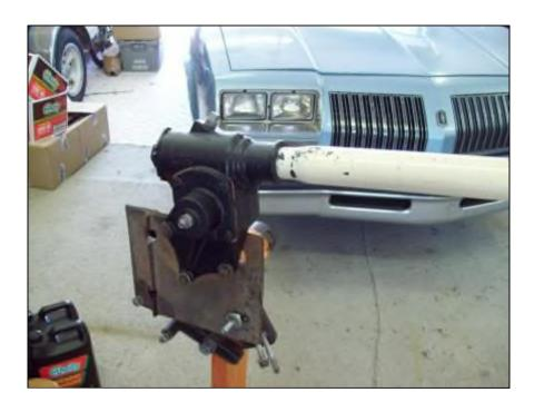
Pump the box full of chassis grease, NOT 80-90wt gear oil.
