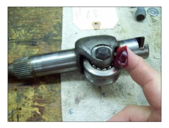
Slide the adjuster, WITH THE SHIM, into the end of the sector shaft.
