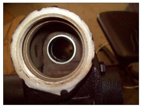
Each end of the worm gear is an inner bearing race. If these race surfaces are damaged or excessively worn, you get to buy an expensive new rebuild kit (the worm IS NOT available separately).
