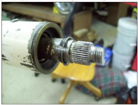
Now, this is when and where the FIRST adjustment is done; **preloading the worm gear bearings.** I place a small pair of vice grips on the splined end of the steering shaft which allows "feeling" the preload of the worm gear bearings. This is done by "experienced feel", not by a service manual procedure.
