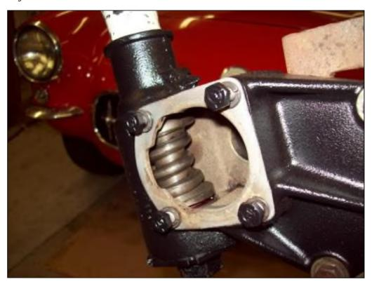
THOROUGHLY pack the ball bearings of the sector roller (on BOTH sides) with grease.
