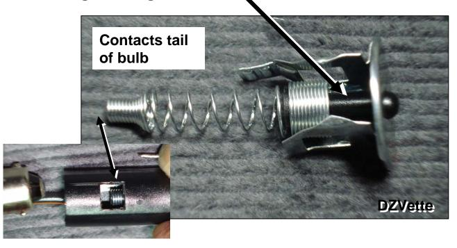
When Glove-box door is open the push button releases the spring which moves forward to make contact with the grounded metal housing closing the circuit to light the lamp.
