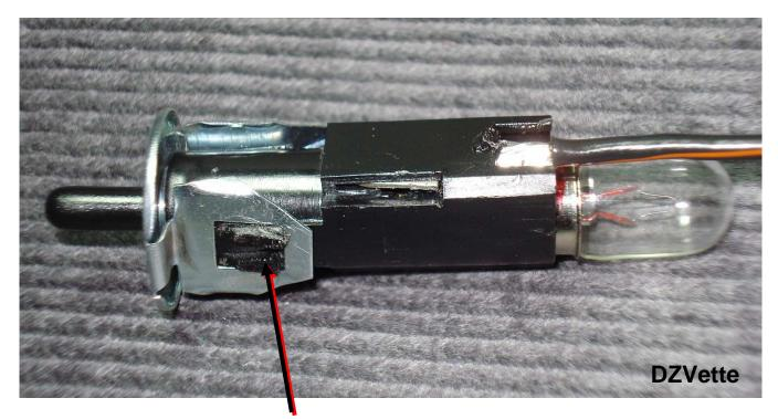
To disassemble the switch trim the melted plastic from this area and gently pry metal side tabs up over remaining plastic. Preserve as much as you can.
