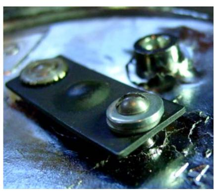
This spring plate presses against the pivot ball in the back of the housing.
